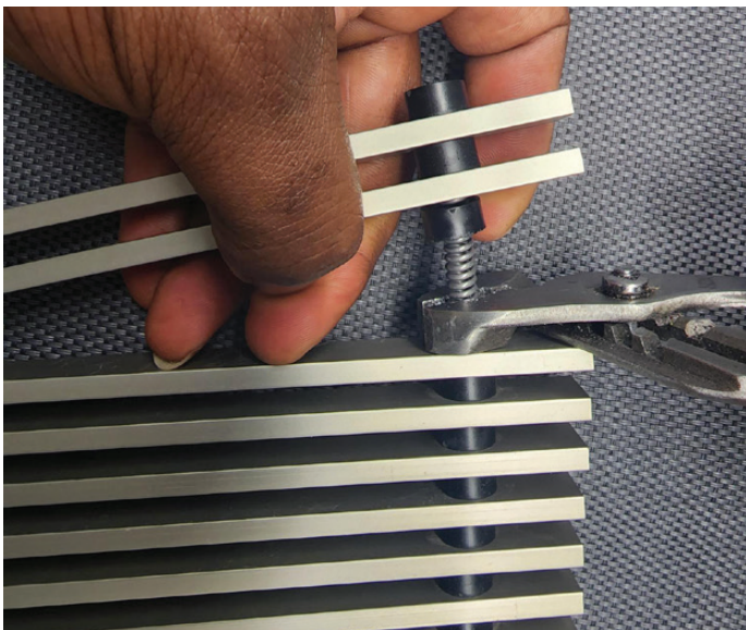
FIGURE 2: POSITIONING LOCKING PLIERS ▼
