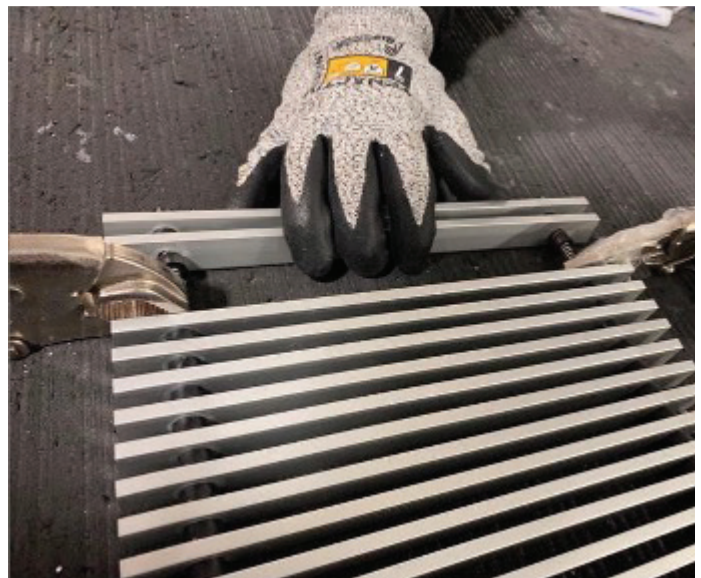
FIGURE 3: FULLY CLAMPED GRILLE ▼
