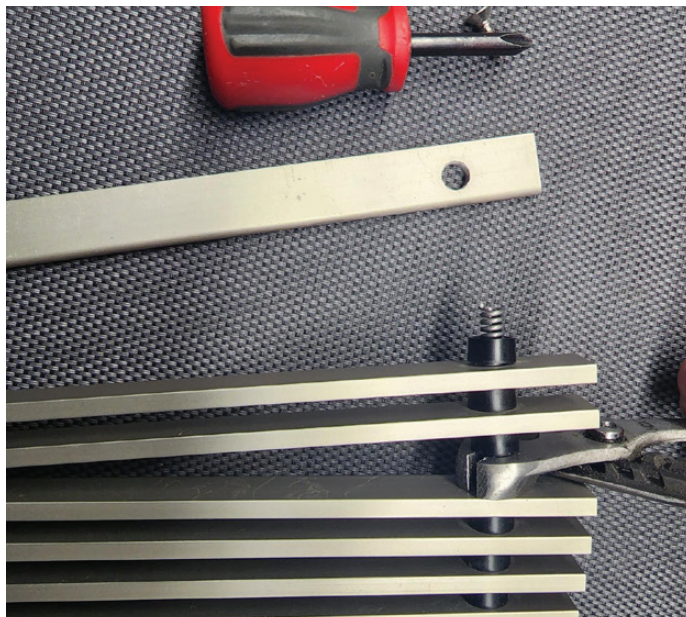
FIGURE 5: REMOVING BARS AND SPACERS ▼
