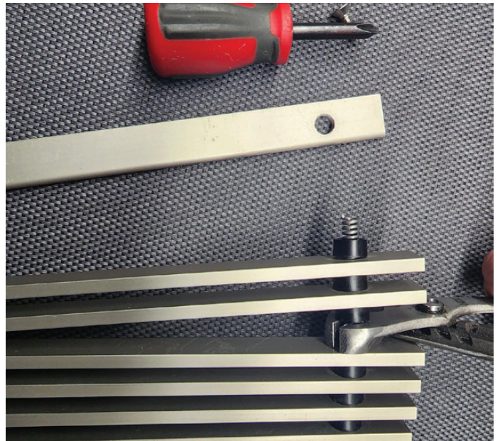
FIGURE 10: ADDING BARS AND SPACERS ▼
