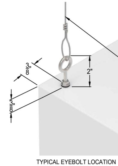
USA SECTIONS TO BE HUNG WITH PRE-STRESSED 12 GA. HANGER WIRE TO SLAB OR STRUCTURAL STEEL ABOVE THE CEILING ACCORDING TO ASTM C636, OR LOCAL BUILDING CODES (AS APPLICABLE)
