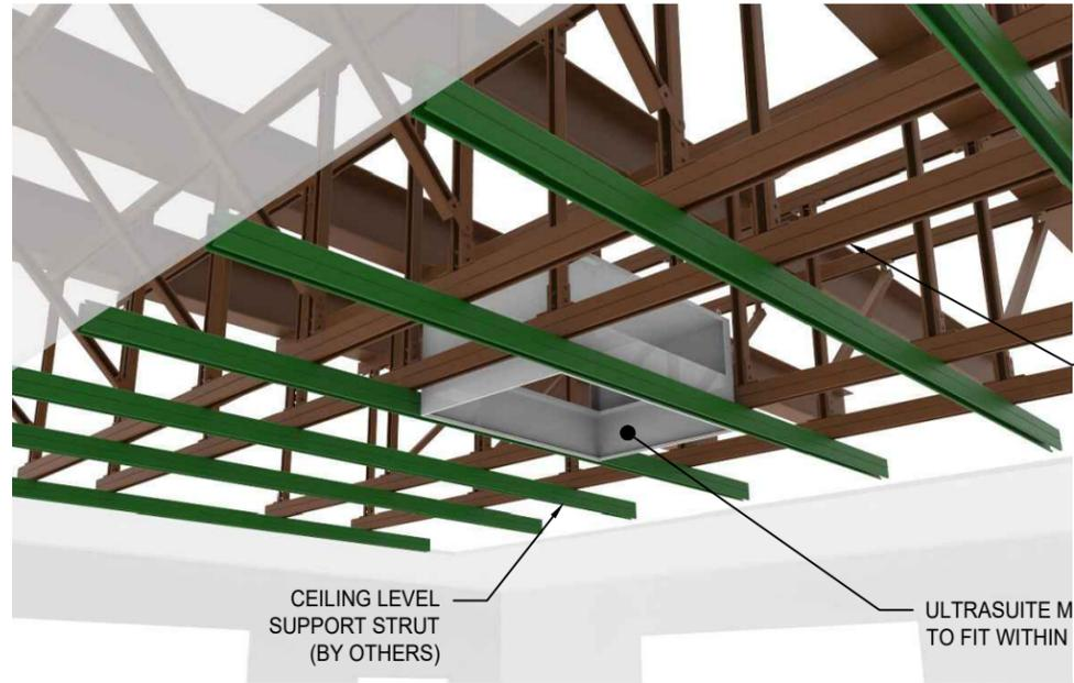
REMOVE INTERNAL COMPONENTS AND RAISE ULTRASUITE MODULES. FASTEN TO UNISTRUT AS SHOWN ON PAGE 10
