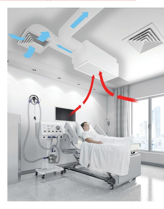
In these applications the Puraflo should be located directly over the patients head so that contaminated air is drawn directly out of the room, and filtered air should be supplied toward the door so that airflow is encouraged to move from clean to less-clean areas of the room.
