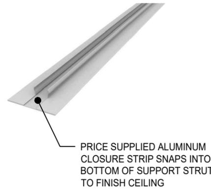
PRICE SUPPLIED ALUMINUM CLOSURE STRIP SNAPS INTO BOTTOM OF SUPPORT STRUT TO FINISH CEILING
