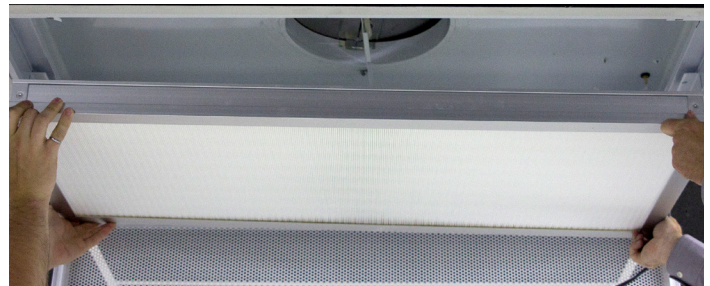
B) ENSURE KNIFE EDGE OF PLENUM SEATS INTO GEL CHANNEL. USE GUIDES TO ASSIST WITH PROPER KNIFE EDGE ALIGNMENT.
