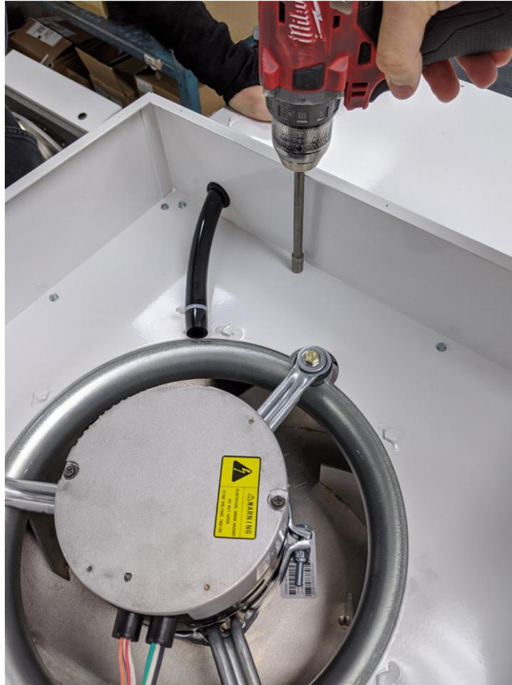
**Step 6:** Remove motor/blower assembly from the inlet collar by removing the 6 lock-nuts using a deep 7/16" socket wrench (or equivalent).
