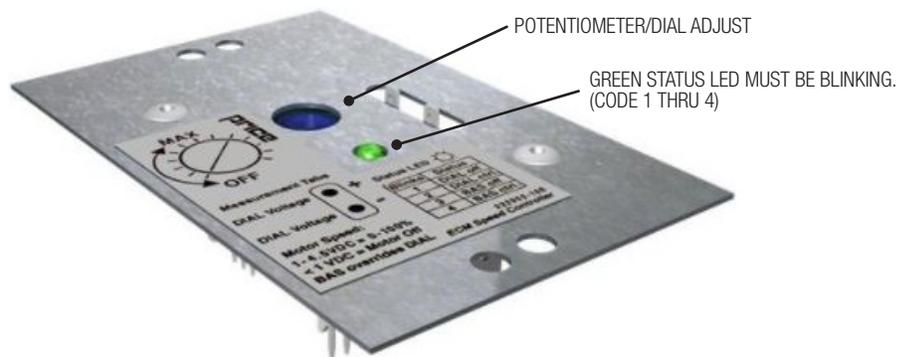
**Step 3:** Wait a few seconds for the ECM motor to adjust its speed and then verify fan airflow with measurements at the unit face using a flow hood. Adjust the POT/DIAL, or BAS input signal to reach desired airflow as required.
