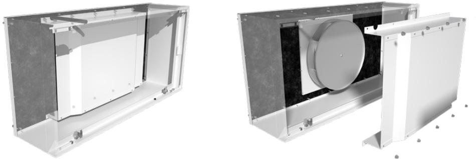
**NOTE:** A 7/16" ratchet with extension is recommended for ease of access for unfastening.
