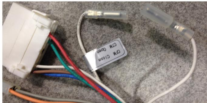
**Switching from constant torque to constant flow:** To switch the motor from constant torque to constant flow all that is required is to close the connection of the white wire as shown.
