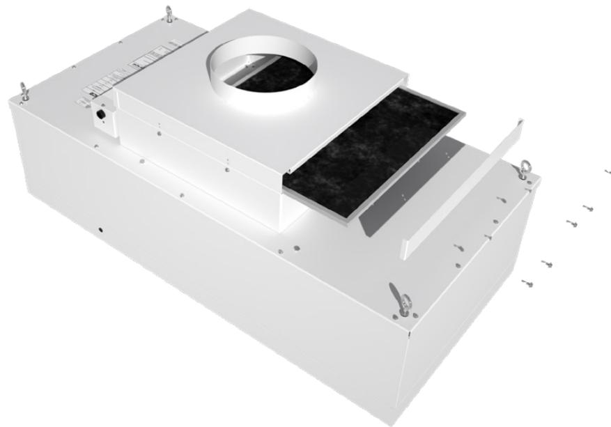
**Step 3:** Clean pre-filter by hand washing in water with a mild detergent or by using a vacuum cleaner. Allow pre-filter to dry completely before replacing.
