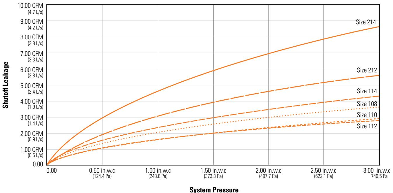
**NOTE:** Casing leaking for VFX is <1.5 CFM (0.7 L/s) up to 3 in.w.c. (746.5 Pa) for all valve sizes.
