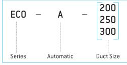
Ceiling diffusers shall be Holyoake Series ECO-A, manufactured from injection moulded tough U.V. stabilised and fire rated engineering polymer, in self coloured white as standard. Series ECO-A shall have the ability to regulate the airflow via an adjustable central cone and automatically direct a portion of the airflow downwards, when supplying air above 30°C. All shall be as manufactured by Holyoake.
