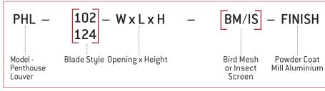
PHL Penthouse Louvers shall be constructed from welded aluminium extrusion with mitred corners. Heavy, extruded aluminium blades and heavy gauge aluminium roof, with bird mesh, or insect screen.
