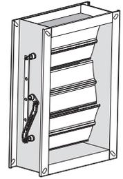
Balancing Dampers shall be of extruded aluminium construction. Frames shall be suitable for duct flange mounting. Blades shall be fixed to 11 mm hexagonal shafts held by two piece acetal self lubricating bearings, with outer shells fluted to prevent rotation.
